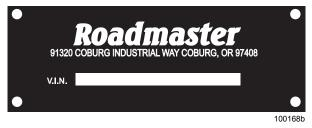
Tag located on curbside frame behind front wheel and in generator compartment.
