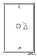
Antenna Boost: Located in passenger side overhead cabinet.
