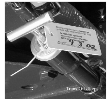
Transmission Oil Level Dipstick.
