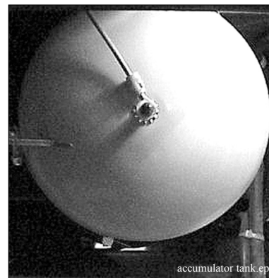
Remove tank valve cap to check air pressure.
