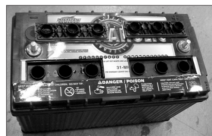
Battery with cover removed. The plastic cover must be cut to be removed.
