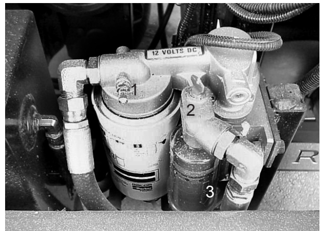
1. Schraeder valve. 2. Thumb screw. 3. Reusable filter.
