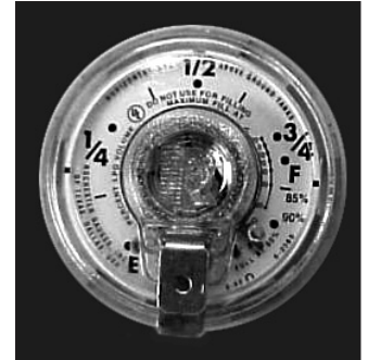
The LP-Gas tank gauge will read 3/4 full when it is filled to capacity.
