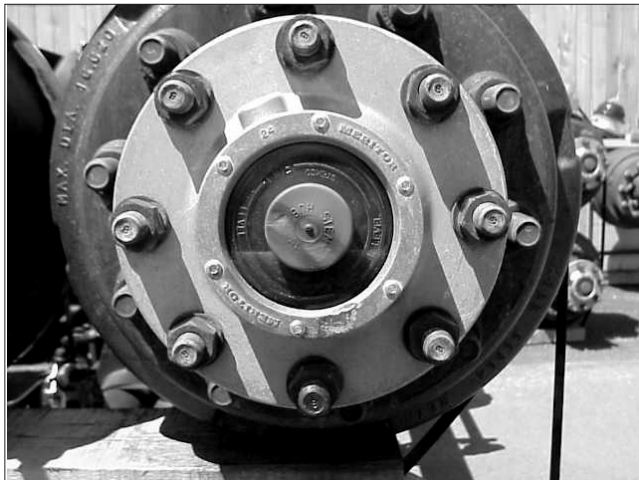
Check the oil level on the tag axle.
