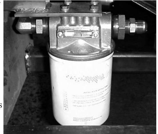
Hydraulic filter for the power steering and hydraulic cooling fans.
