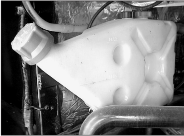
The coolant capacity, when changing the antifreeze, is approximately 11½ gallons.
