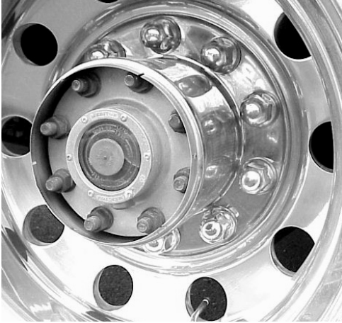
Remove the center hub cap to inspect the tag axle oil level.
