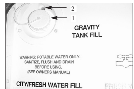
1. Gravity Tank Fill. 2. Vent.
