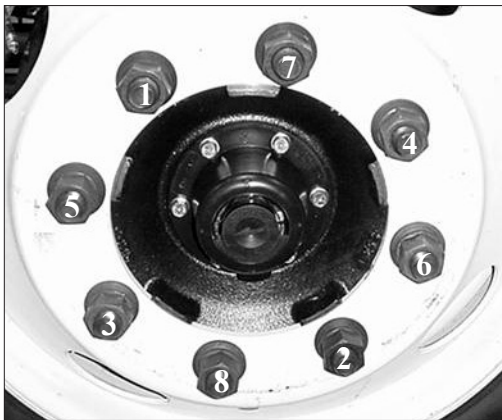
Lug nut tightening sequence.
