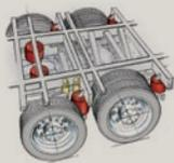
Unique three-degree rear axle tilt perfectly aligns the engine, transmission and differential, minimizing stress on the drivetrain and reducing noise in the coach.
