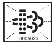
DPF light & warning alarm 090502a
