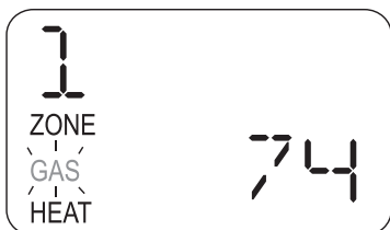
Example of heat pump screen in backup furnace mode. 031359a
