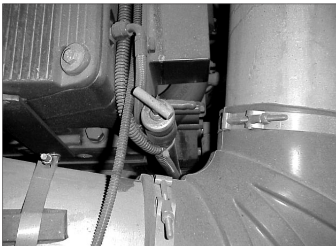
Transmission Oil Level Dipstick.
