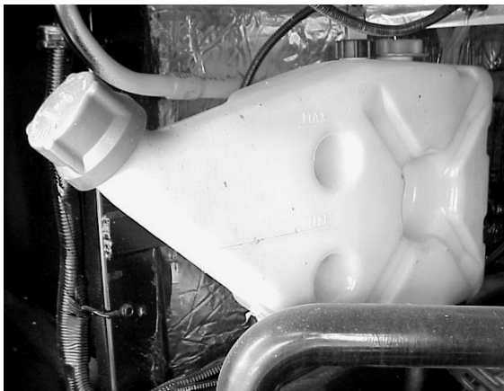
The coolant capacity, when changing the antifreeze, is approximately 11½ gallons.
