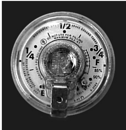
LP Tank Gauge
